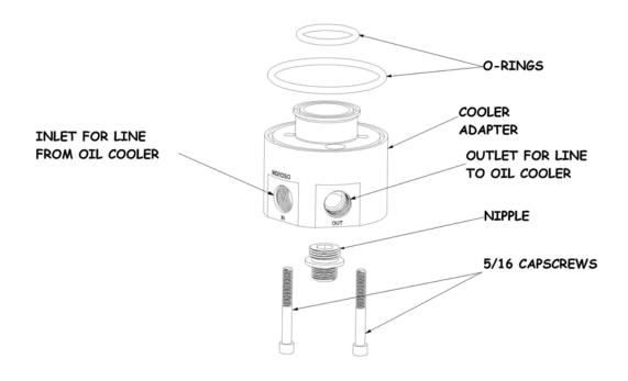
Remove factory oil filter adapter from engine. Assemble components as shown in the above illustration. Make certain to use #10AN fittings and o-rings to plumb your oil cooler. This adapter has no bypass valve for the oil filter.
