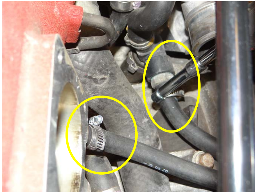
Step 2: Locate and remove 3/8" lines that run to intake and PCV Valve.
