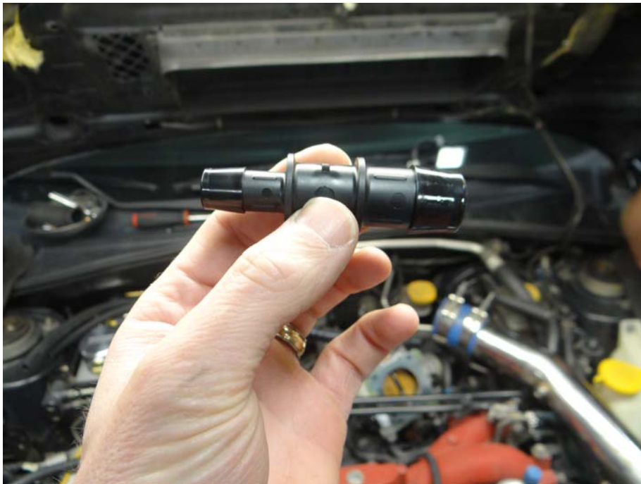
Step 8: Install \frac{3}{4} to \frac{1}{2} coupling into crank case vent tube.
