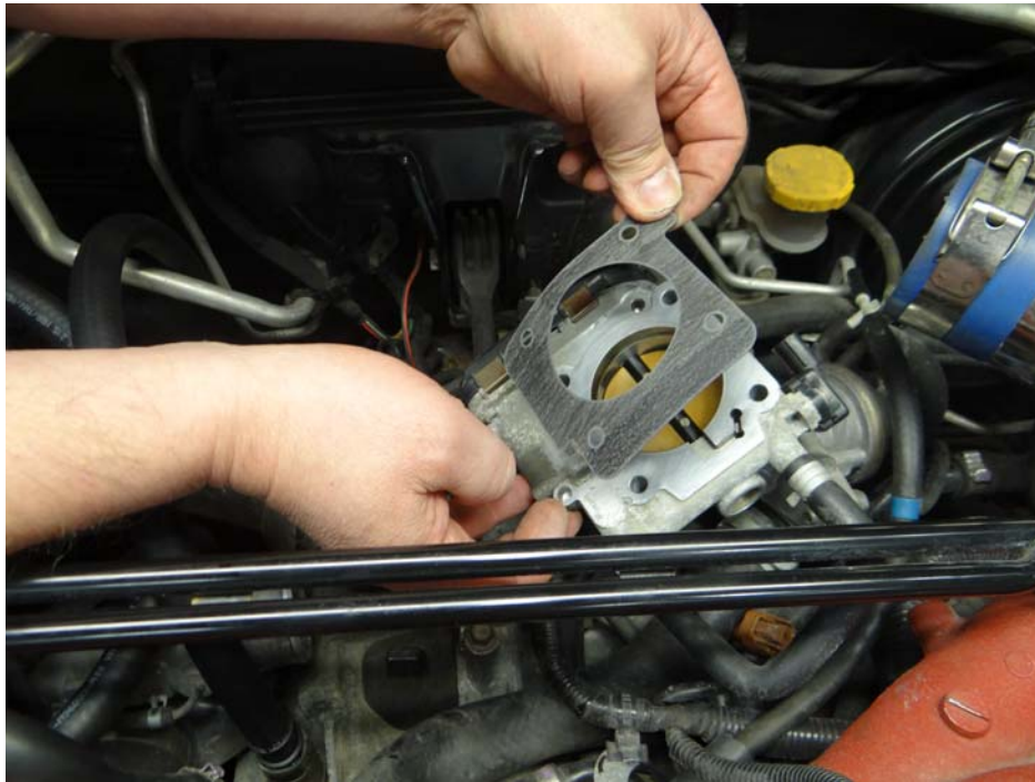
Step 15: Install new throttle body gasket and re-install throttle body. For Technical Assistance, call Moroso's Tech Line (203)-458-0542, 8:30am-5:00pm Eastern Time MOROSO PERFORMANCE PRODUCTS, INC.
