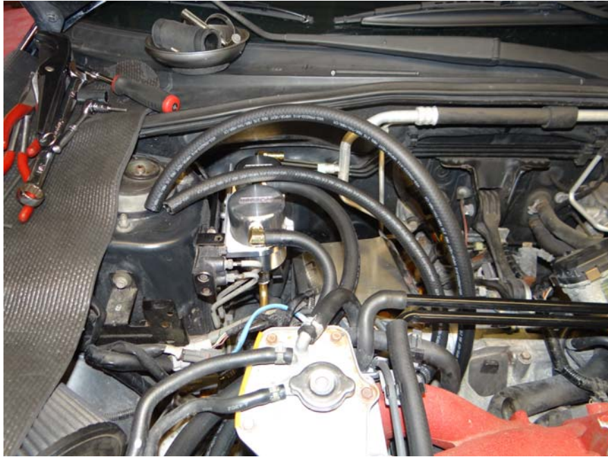
Step 14: Route ½" hose to Air Oil Separator.
