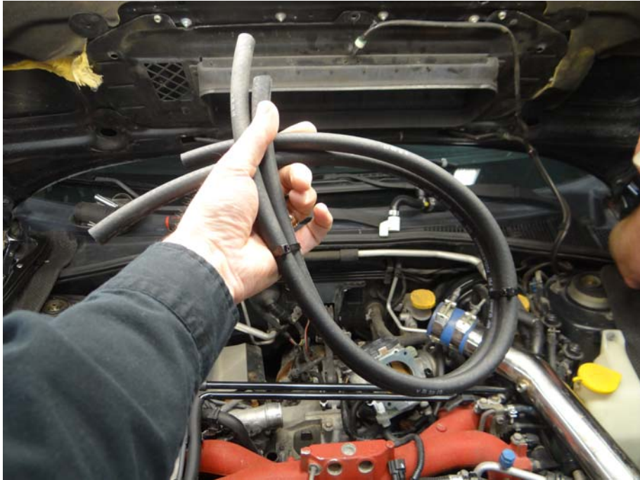
Step 10: Remove 3/8 lines from Air Oil Separator and discard.
