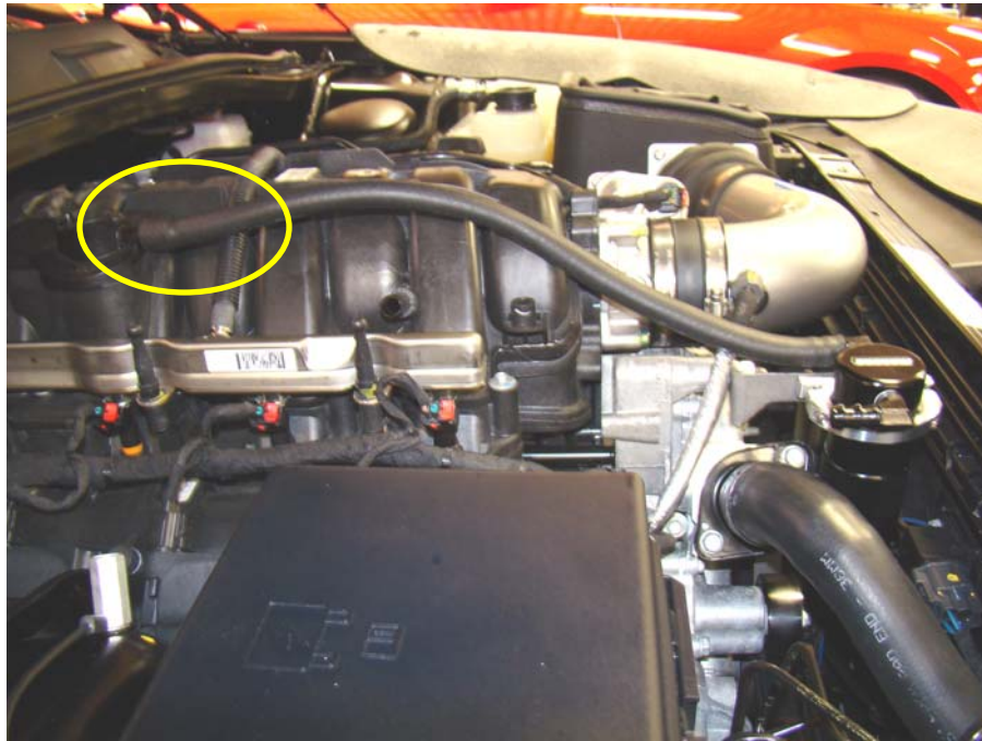
Step 9: Insert other end of hose over PCV nipple as shown.
