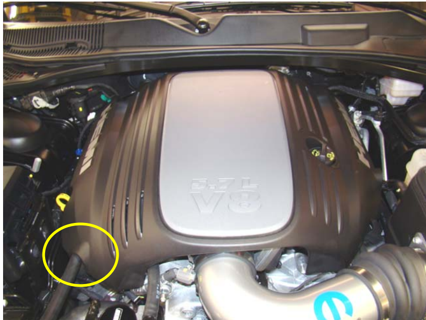
Step 11: Re-install engine cover and route hose to Air Oil Separator.
