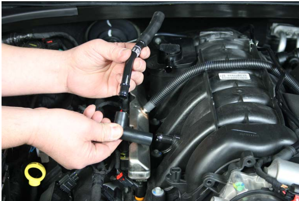
Step 2: Locate and remove PCV line from vehicle.
