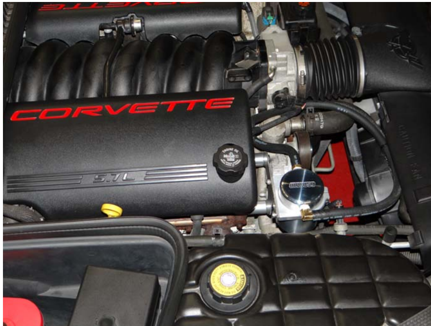
Step 18: Re-install engine cover and oil fill cap. Installation Complete.
