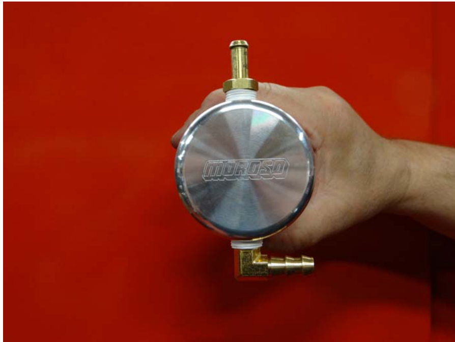
Step 10: Assemble Air Oil Separator as shown using Teflon tape on fittings.
