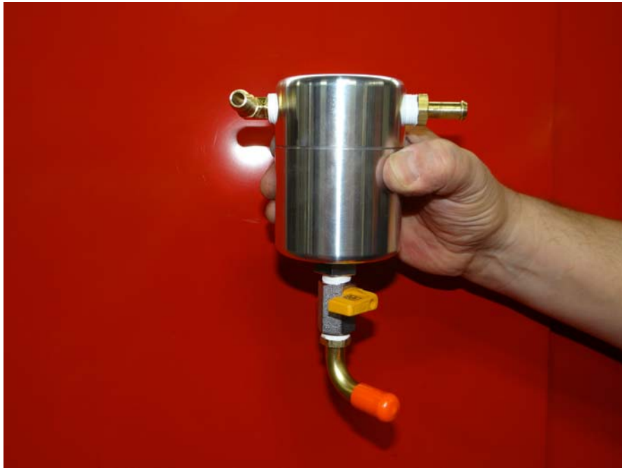
Step 11: Assemble Air Oil Separator as shown using Teflon tape on fittings.
