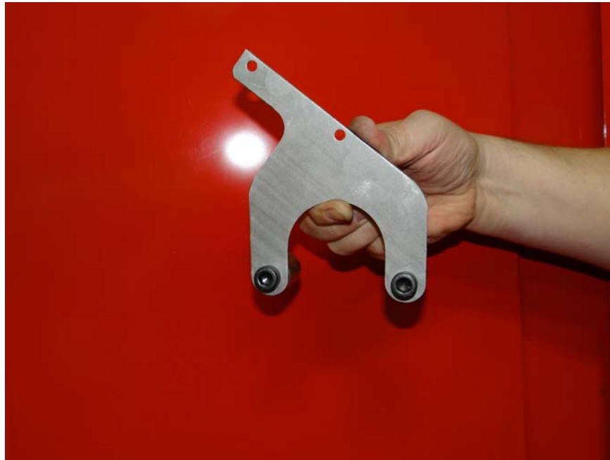
Step 7: Assemble stainless steel bracket as shown in above and below illustrations.
