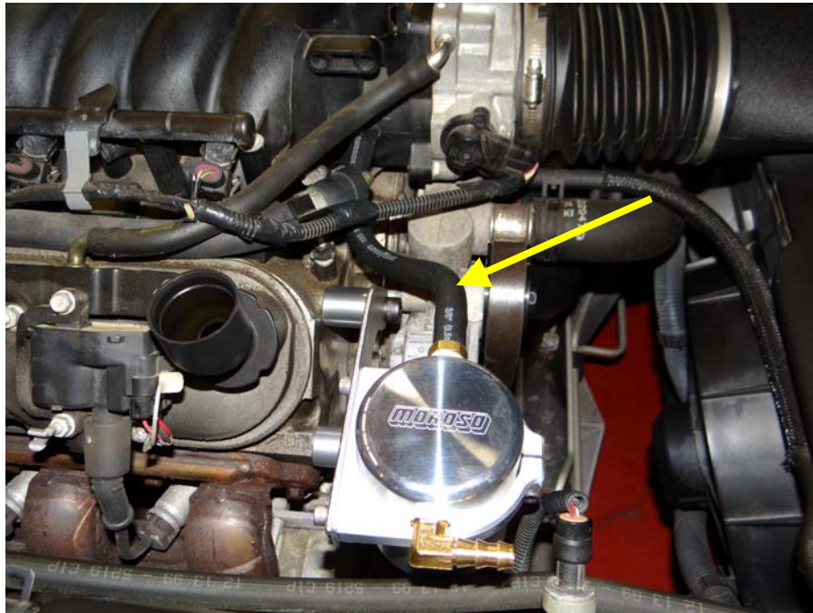
Step 15: Route other end to Air Oil Separator as shown and install to straight fitting.
