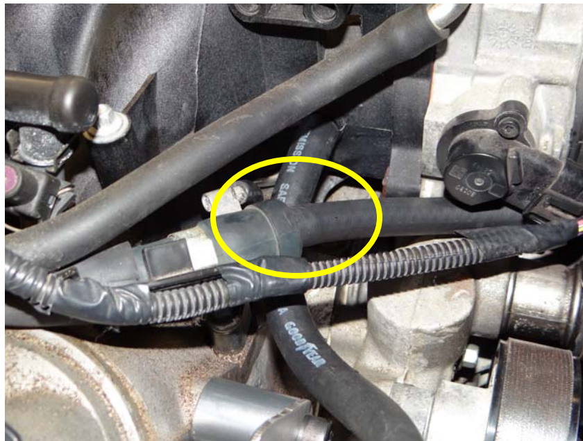
Step 16: Install 27" length of hose to PCV nipple.
