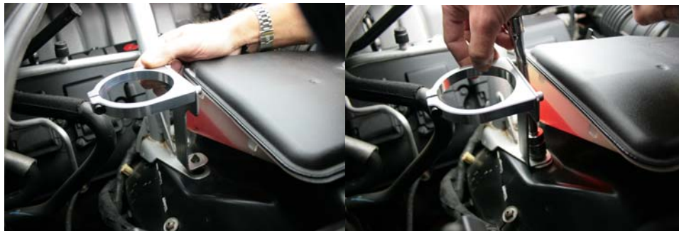
Step 4 Install and tighten billet / stainless bracket as shown to strut tower stud.
