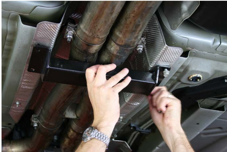
Step 2; Install floor pan brace using stock hardware. Installation complete
