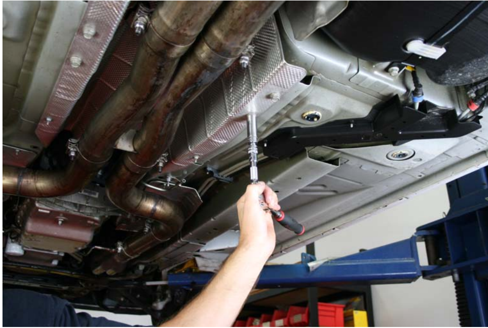
Step 1: Remove tunnel mount bolts and stock brace if equipped.
