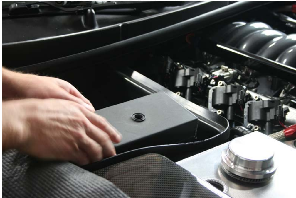
Step 7: Reinstall stock fuse box cover
