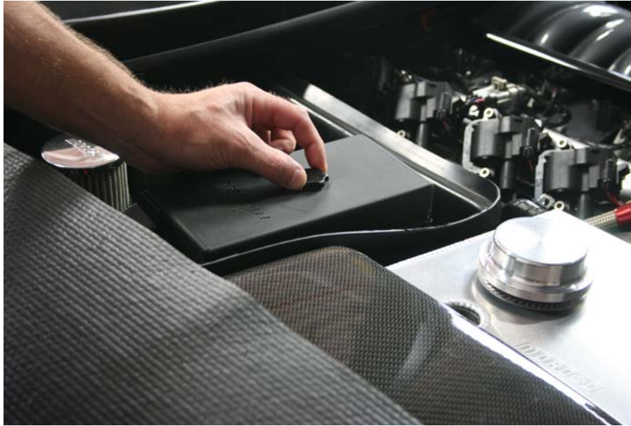
Step 1: Remove fuse box cover hold down screw
