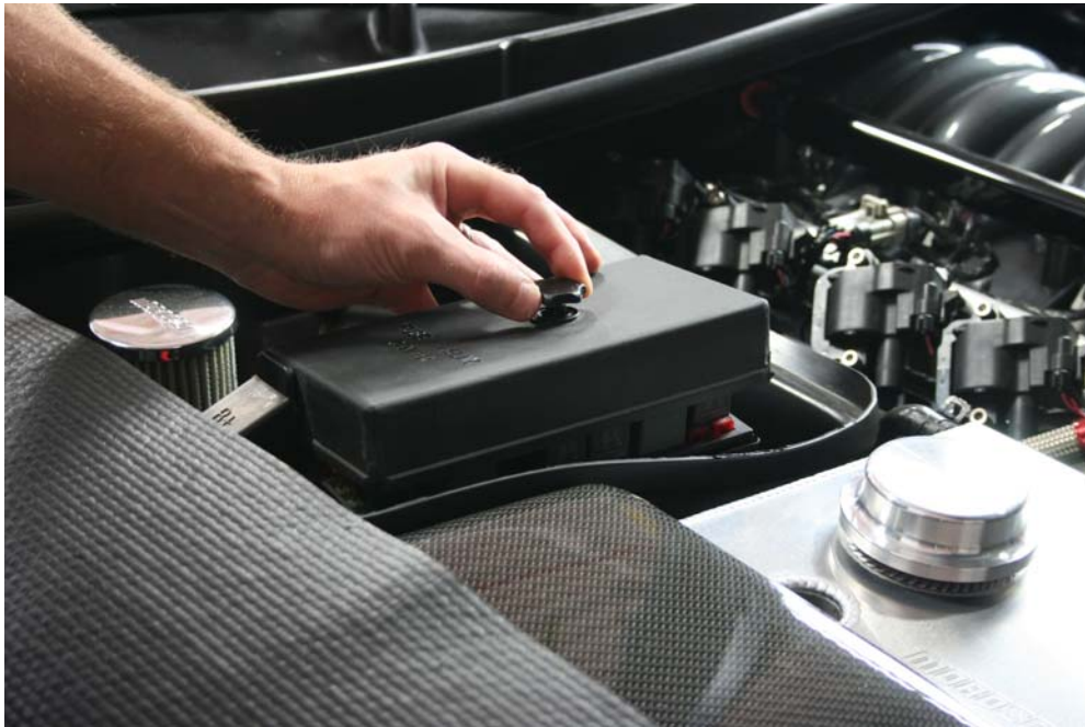
Step 2: Remove fuse box cover
