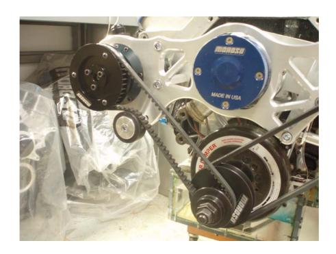
AN ALTERNATIVE TO THE V-BELT FOR THE VACUUM PUMP WOULD BE TO USE A RADIUS TOOTH SETUP. MOROSO OFFERS SEVERAL PART NUMBERS FOR THIS INSTALLATION. THE PULLYS ARE, 23540 FOR THE VACUUM PUMP AND, 23533 FOR THE CRANKSHAFT. ANY ONE OF THE THREE FOLLOWING BELTS CAN BE USED. MOROSO PART NUMBER 97151 (760MM), 97152 (776MM) OR, 97154 (800MM).
