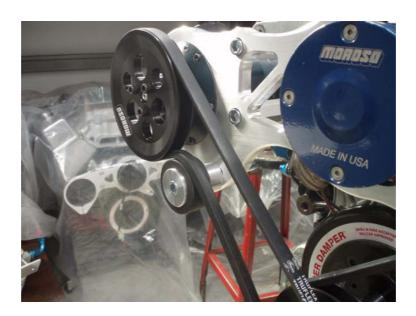
ENSURE THAT THE PULLEYS ARE IN ALIGNMENT. SWAPPING SPACERS ON THE DRIVE MANDREL CAN MAKE BIG ADJUSTMENTS. MOVING THE PUMP WITHIN THE BRACKET CAN DO MINOR ADJUSTMENTS.
