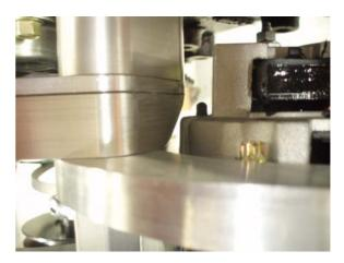
USING THE FOUR 3/8 X 1.000" SOCKET CAPSCREWS, ATTACH THE MAIN BRACKET TO THE STANDOFFS. DO NOT TIGHTEN AT THIS TIME, JUST START A COUPLE OF THREADS AND LET THE BRACKET HANG FOR NOW.
