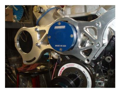
ONCE THE FOUR SOCKET CAPSCREWS ARE STARTED, GO BACK AND TIGHTEN THE FOUR STANDOFFS WITH A 3/4" WRENCH. LEAVE THE FOUR CAPSCREWS FINGER-TIGHT UNTIL YOU HAVE THE ALTERNATOR MOUNTED.
