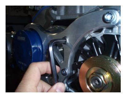
THE KIT PROVIDES BOTH AN 8MM AND A 3/8" FASTENER FOR THE LOWER LUG ON THE ALTERNATOR. THE ALTERNATOR IS TAPPED FOR 8MM THREADS SO, THE MATCHING FASTENER CAN BE USED AT THIS TIME TO COMPLETE THE INSTALLATION. FOR THOSE WHO WISH TO CONVERT TO A 3/8" BOLT, THE ALTERNATOR MUST BE DRILLED OUT. USE CARE AND MASK OFF ALL OPENINGS TO INSURE NO FOREIGN MATTER GETS INTO THE ALTERNATOR.
