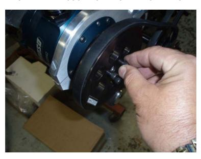
\*ANY V-BELT WITH A 4L CROSS SECTION AND A MINIMUM LENGTH OF 33 INCHES (4L330) TO A MAXIMUM LENGTH OF 34.625 INCHES (4L346) CAN BE USED TO DRIVE THE VACUUM PUMP.
