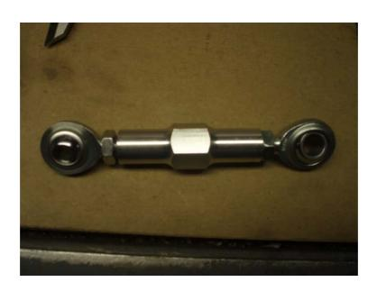
ASSEMBLE THE LOWER ADJUSTER BY THREADING THE JAM NUTS ONTO THE ROD ENDS, AND THEN THREADING THE ROD ENDS INTO THE ADJUSTING LINK.
