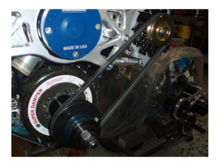
PLACE THE VACUUM PUMP, MINUS PULLEY, THROUGH THE BACK OF THE INSTALLED BRACKET. IT SHOULD FIT WITH A LIGHT PRESS AND ROTATE FREELY WITHOUT THE PINCH-BOLT TIGHTENED.
