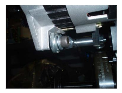
ONCE THE ADJUSTING LINK IS SECURED, THE DRIVE BELT CAN BE INSTALLED. TURN THE ADJUSTING LINK SO THAT IS AT IT'S SHORTEST LENGTH (ALTERNATOR TOUCHING WATER PUMP). WITH THE RECOMENDED 4.000 CRANK PULLEY (MOROSO PART#23523) INSTALL EITHER A 4L318 (31 ¾") OR A 4L320 (32") V-BELT (BOTH WILL WORK). ADJUST LINK TO ACHIEVE PROPER TENSION AND TIGHTEN BOTH JAM NUTS AND THE UPPER AND LOWER BOLT.
