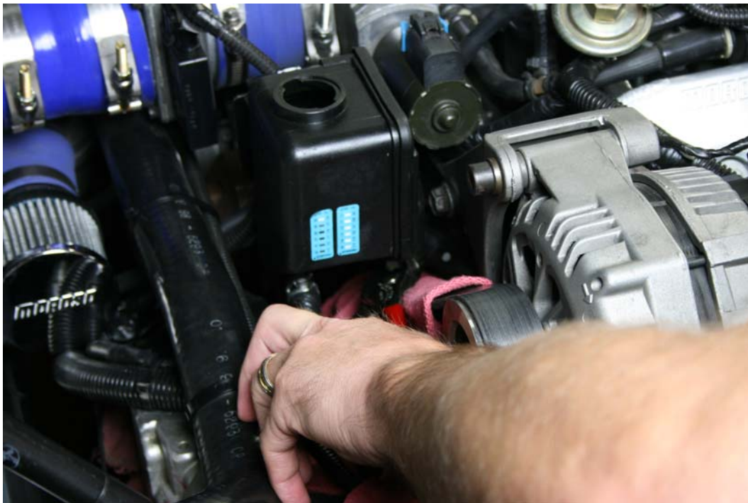
Step 2: Slide rear hose clamp down from tank
