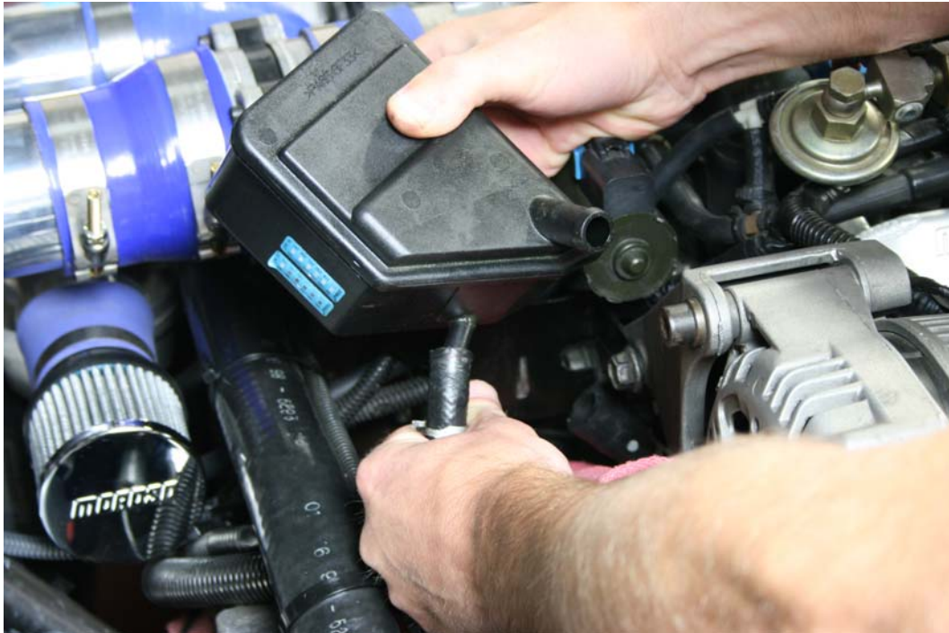
Step 6: Remove front line from tank
