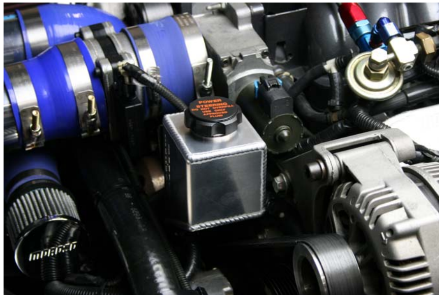
Step 11: Fill with fluid and reinstall fill cap
