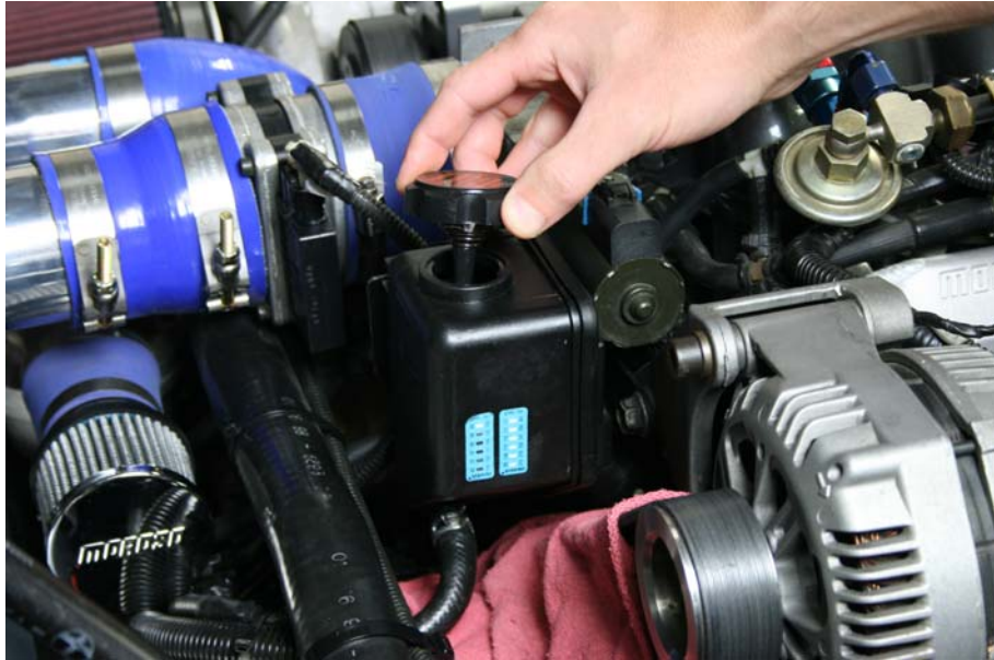
Step 1: Remove power steering cap, remove as much fluid from tank as possible
