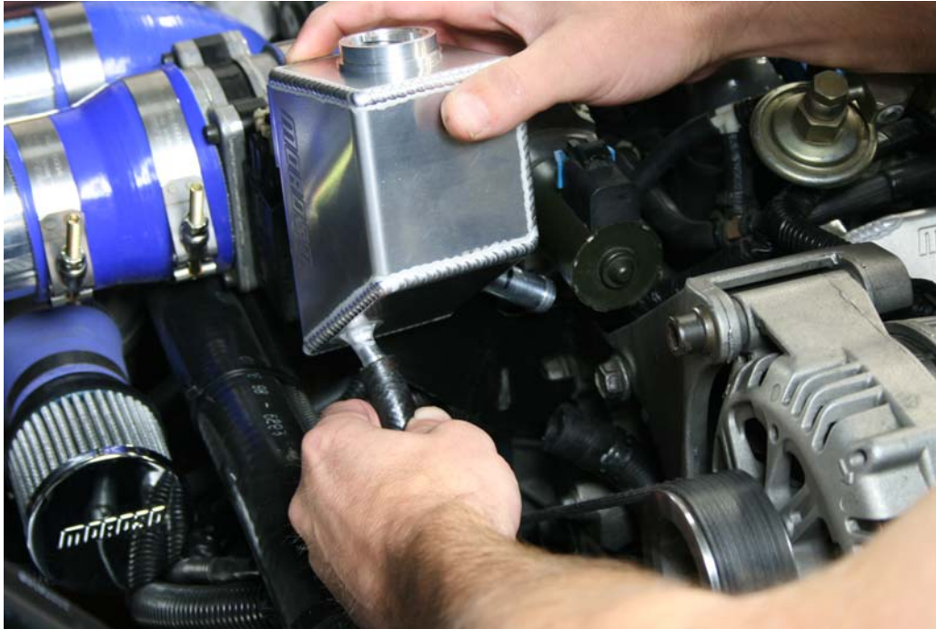
Step 7: Install front line over nipple
