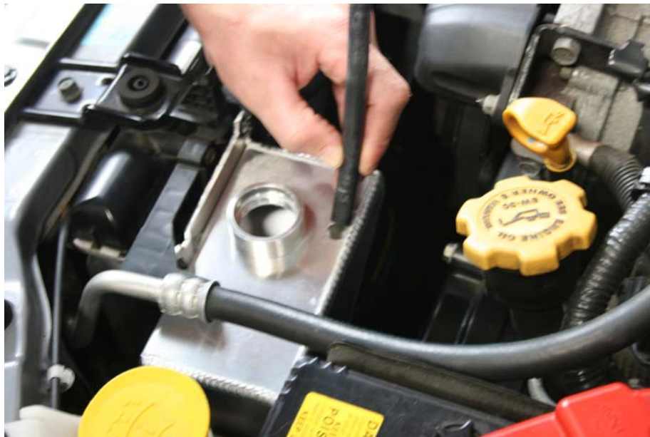
Step 10: Insert siphon tube into coolant tank
