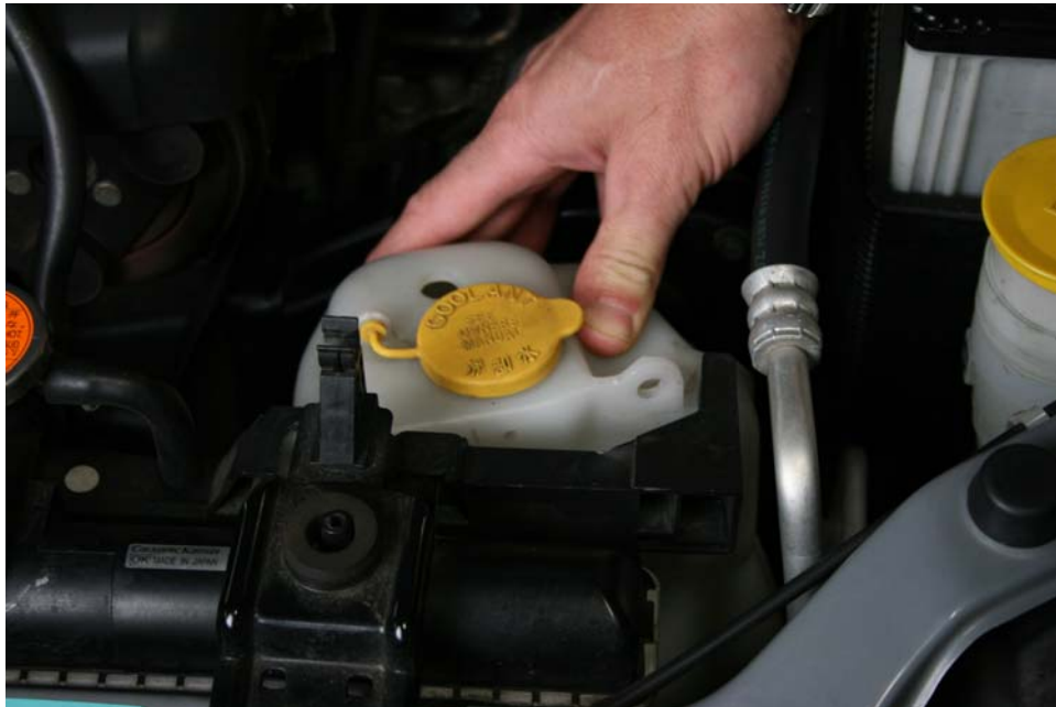
Step 3: Release hold down tab and twist tank to remove from mount
