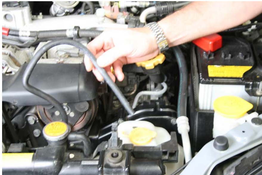
Step 2: Remove Siphon Hose from Coolant Tank
