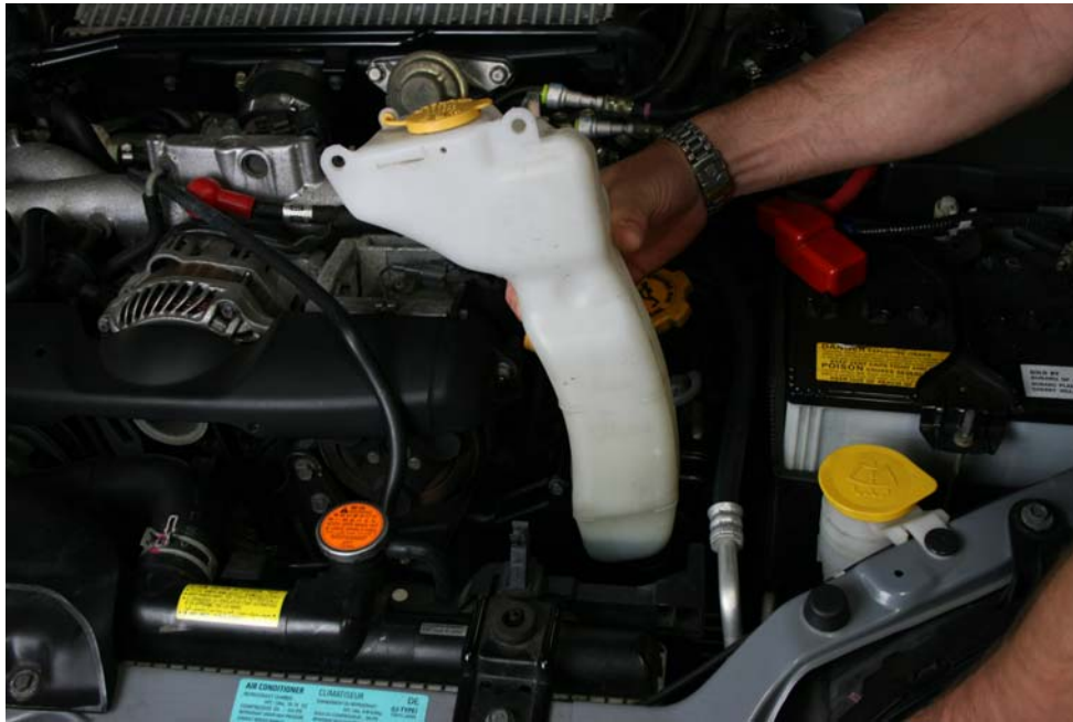
Step 4: Remove Coolant Tank from vehicle
