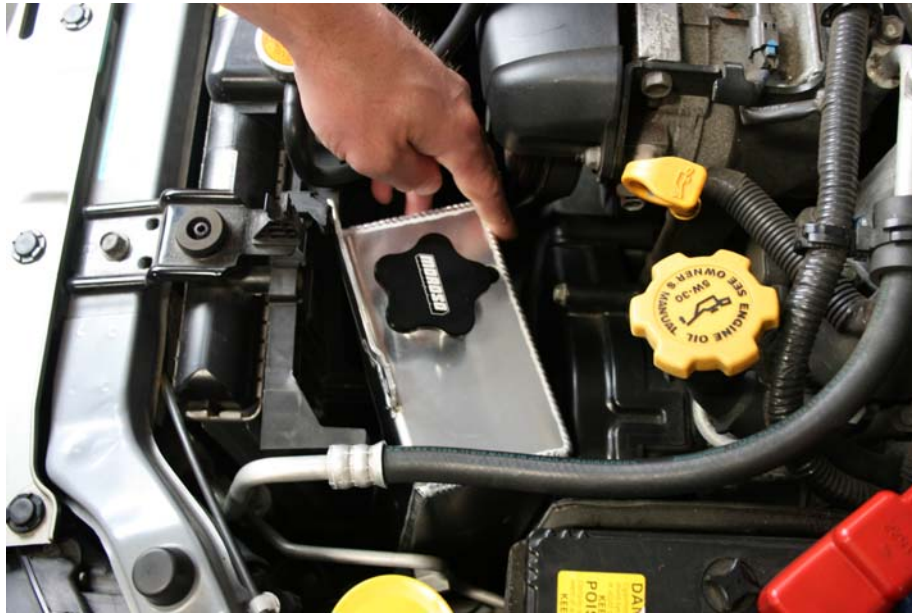
Step 6: Insert lower mount into bracket (on bottom of coolant tank)
