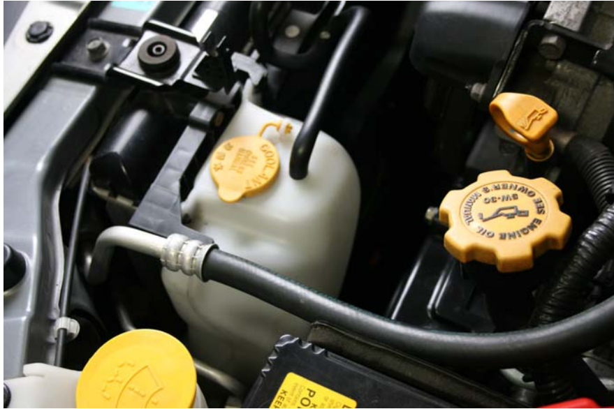
Step 1: Locate Coolant Tank
