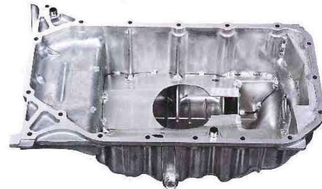
Trap doors and baffle plates help to keep oil from sloshing away from the oil pickup.
