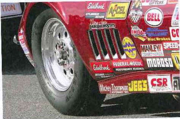
(Above) Lighter is better, so drag racers use skinny front tires that save weight, have a small contact patch, and provide the potential for less drag when aired up.
