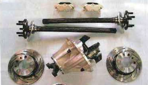
Reducing weight in the driveline cuts parasitic drag and helps the vehicle accelerate faster. Pictured are some parts from Strange, including gun-drilled axles, lightweight calipers and rotors, and a back-cut ring gear.
