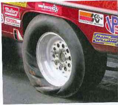
Most stick racers rely on bias-ply tires, which are run at relatively low pressure. This allows them to absorb the shock from the initial hit during launch but creates lots of drag downtrack.
