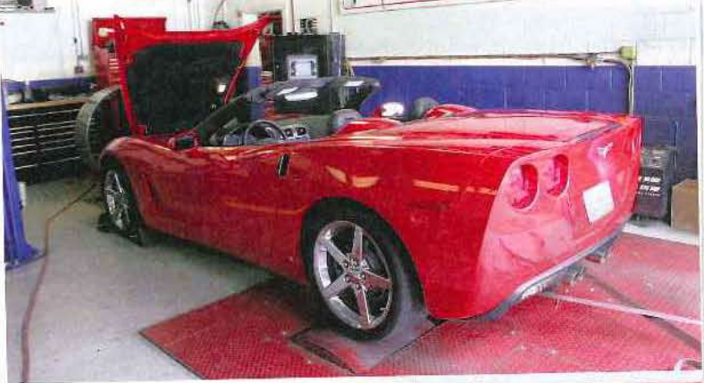
You can find gains in performance by testing on an engine or chassis dyno. I've seen gains of 5 to 10 horsepower at the wheels just by changing tire compounds.
