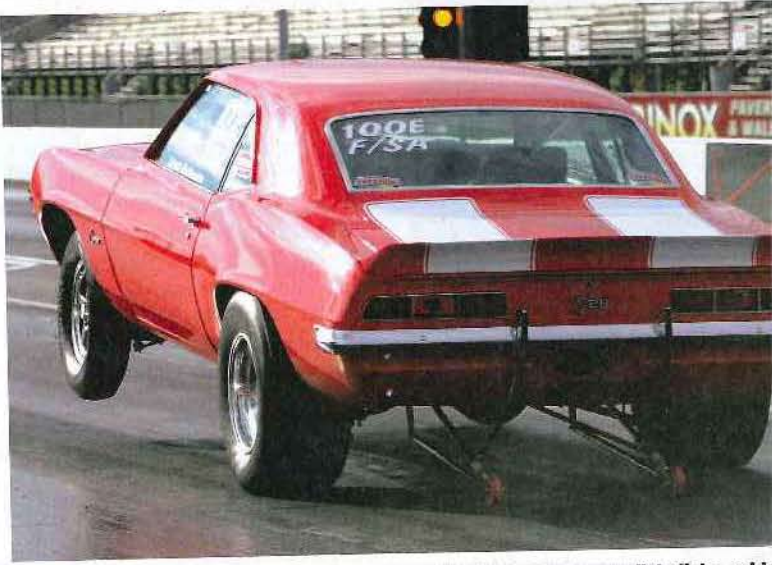
In contrast, many automatic racers use radial slicks, which are much stiffer and thus have less drag. This is one reason they are quicker in back-to-back testing than bias-ply tires
