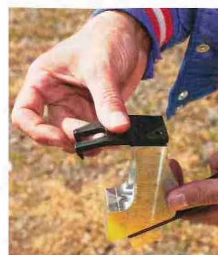
Each claw can be interchanged easily on the Moroso tool with the use of a wing nut that unscrews and two dowel pins to line each claw up on the aluminum foot.
