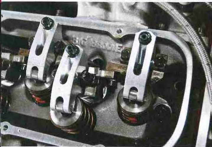
Dollar for dollar, valve springs are probably the most expensive part per cycle in your engine. They tend to take quite a bit of abuse when you think in terms of them going up and down several hundreds of thousands of time during a run.
