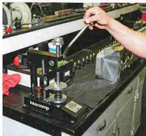
It all starts with checking the valve springs on a bench tester for seat pressure and coil bind. The coils of a spring should never contact one another, which is a sure recipe for damage to any number of components.
