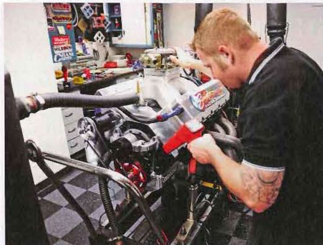
In the case of our engine, Dennis made several changes to the ignition timing to bring the power up to the levels it needed to be.
