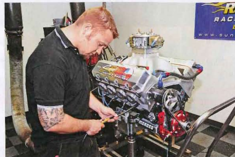
Once dyno testing is complete, Sunset has the confidence the engine will run as planned without any problems. Before the engine is crated up for shipping, Dennis rechecks valve adjustment and performs a leak-down test on each cylinder. The oil is drained and the engine crated for shipment.
