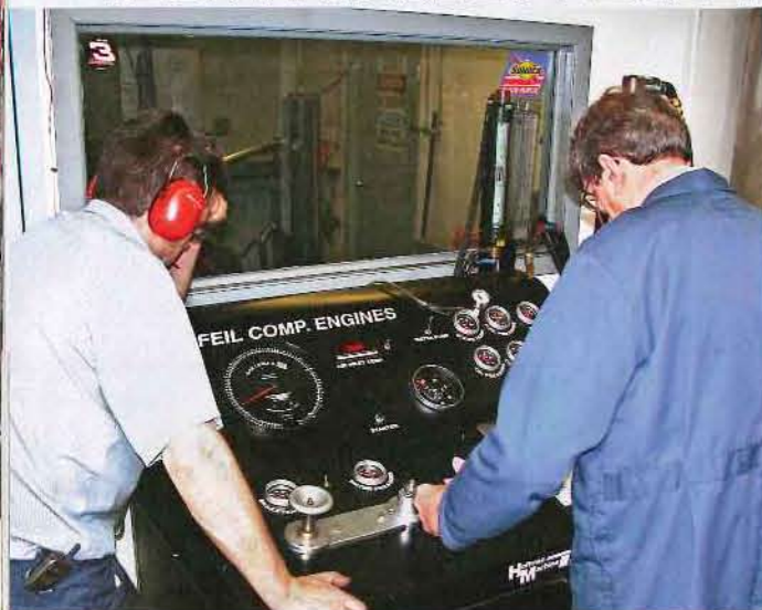
Different from today's computerized dynos, a dyno of old utilized a manually operated water valve which controlled flow to an absorption unit that held an engine to a certain rpm. Oftentimes, it took two people to run the unit.
