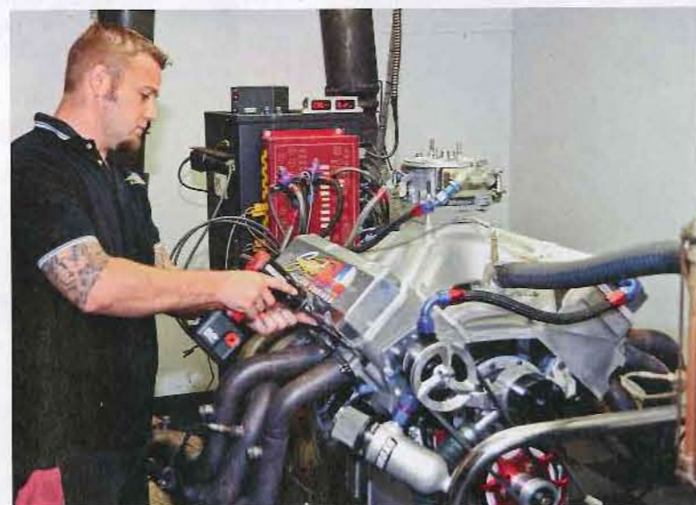
The proper break-in procedure of a new engine is mandatory if you expect good results. Sunset Racecraft's Jason Dennis said, "We run a new engine at 1,800 rpm with just a slight load from the dyno for two 10-minute periods. We then pull the valve covers, run the valves and take apart the System 1 oil filter to inspect for any debris."
