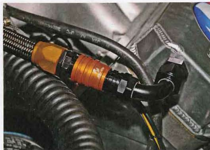
Vacuum pumps allow for negative crankcase pressure but also have a tendency to pull oil away from engine components that rely on splash oiling like wrist pins, lifters, etc. During break-in or even warm-ups, we use a Jiffy-Tite quick-connect fitting with no internal valves to disconnect the pump. final dyno sheet on our 598-inch engine shows 1,224 horsepower and 909 ft.-lbs. of torque. Next step is on-track testing.
