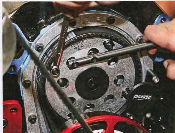
The beauty of running an engine on a dyno is that you eliminate any of the variables of on-track testing. Items such as camshaft timing can easily be changed and then evaluated without the worry of waiting in line for a run or changing track conditions.
