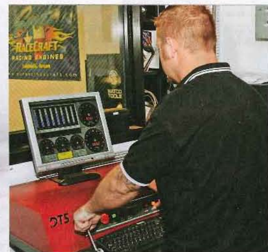
Dyno testing of engines has become the norm not only in the search of horsepower and speed, but also for reliability and longevity. With our Project 598-inch engine complete, it was time to see just what the sum of all its components would add up to.
