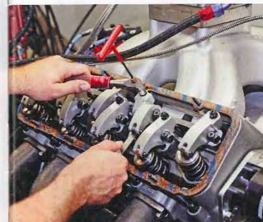
With the engine properly broken in and the oil and water temperature up, the valve adjustment is easily reset with the Jesel shaft rocker system.
