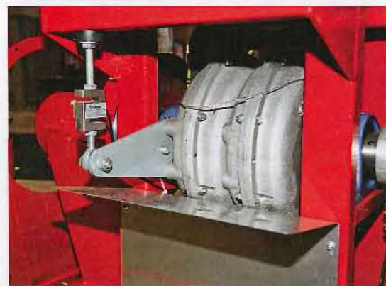
While different brand dynos vary, this is a photo of an absorption unit. Inside the housing resides a rotor. Water flows against the vanes of the rotor to control engine rpm when the carburetor is wide open. The load cell on the left measures resistance to the housing and provides the info to the computer to calculate torque and horsepower.
