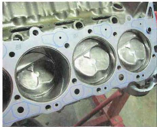
JE pistons will give the big-block 12:1 compression.
