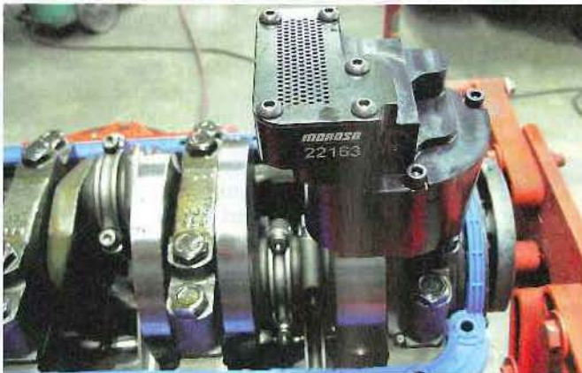
A punched-out 454 (.060-inch over) will power the Nova (hopefully into the high nines).
